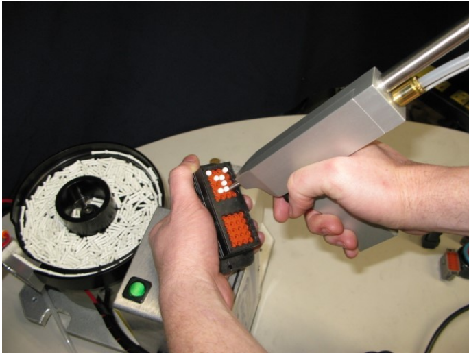
Pictured: CDSS SPG System for TE 114017 (Deutsch size 16) "Large White" Seal Plugs, often used in Automotive Wire Harnesses.
