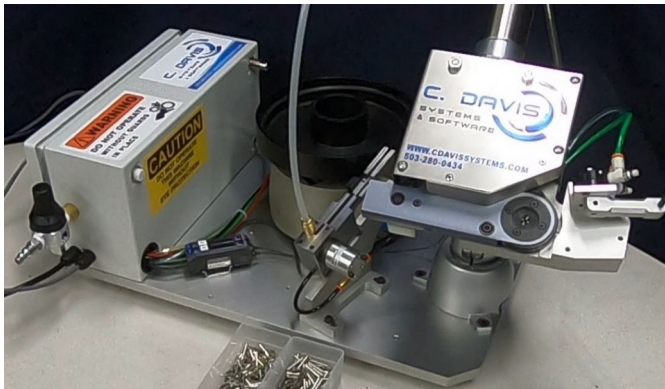
(Pictured: Custom LC Machine featuring Deutsch HDT-40-00 Crimp Tool and Rotary Contact Stopper, with optional Machined Stainless Steel Escapements, Machined Aluminum Parts Bowl.)
